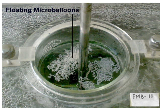
Fig.2: In-vitro buoyancy of floating microballoons
