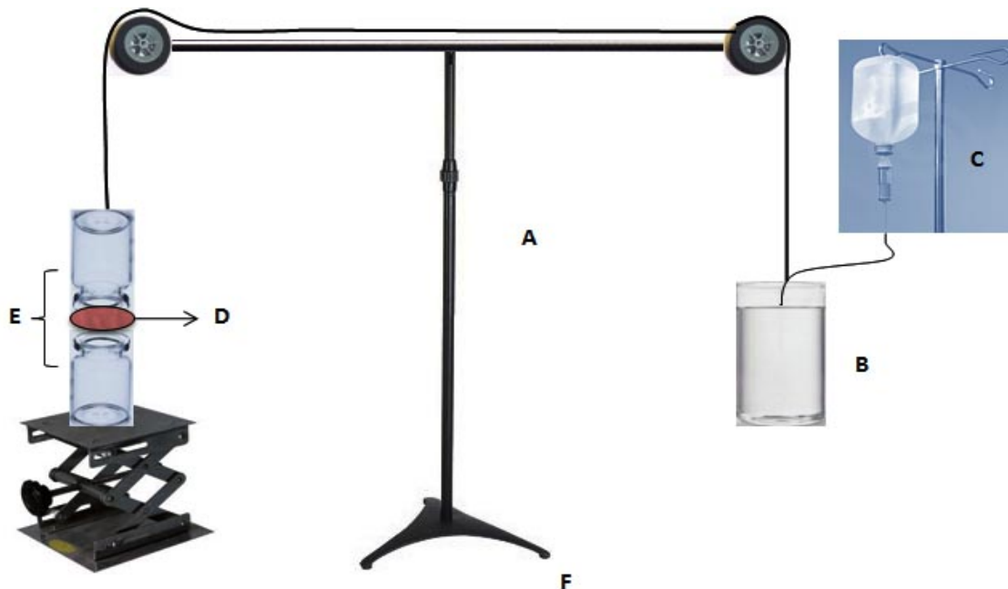
(A) Modified Balance (B) Glass Reservoir (C) Infusion Device (D) Membrane (E) Vial (B) Height Adjustment Pan.
