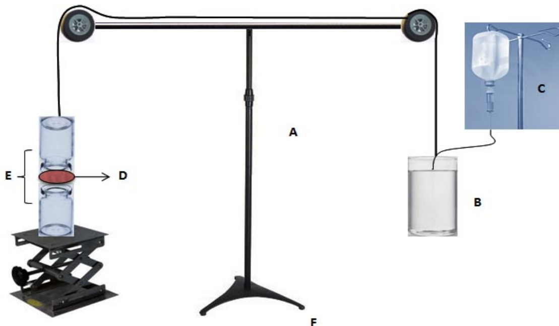
(A) Modified Balance (B) Glass Reservoir (C) Infusion Device (D) Membrane (E) Vial (F) Height Adjustment Pan.
