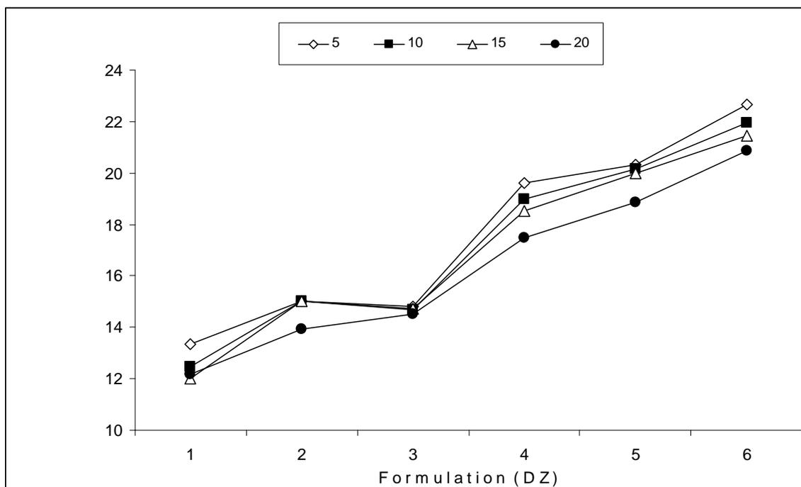
**Figure 6:** Effect of (k) release constant on Higuchi diffusion model for diltiazem formulations compressed at different compression force 5, 10, 15 and 20 kN
