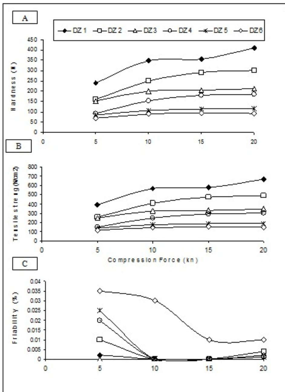
**Figure 1:** Relation between compression force and each of A- Hardness, B- Friability, and C- Tensile strength for diltiazem formulation compressed at 5, 10, 15 and 20 kN.
